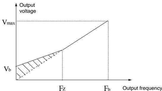
Vb: Manual torque boost                      Vmax: Max. output voltage
