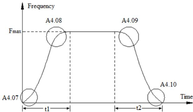
Fig.6-14 Acc/Dec starting time and ending time
