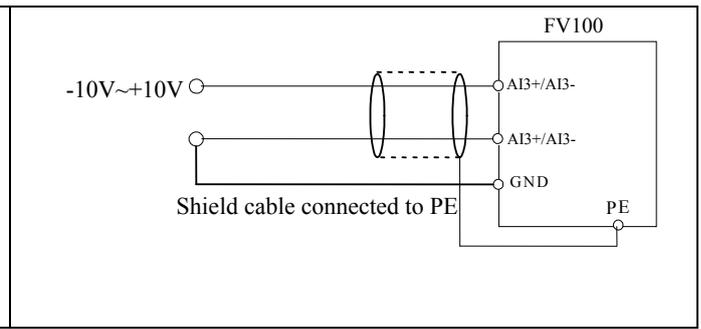
Fig 4-5 AI+, AI- single-ended voltage input wiring
