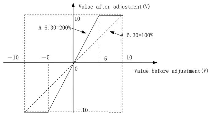
Fig.6-31 Relationship curve between analog output and gain
