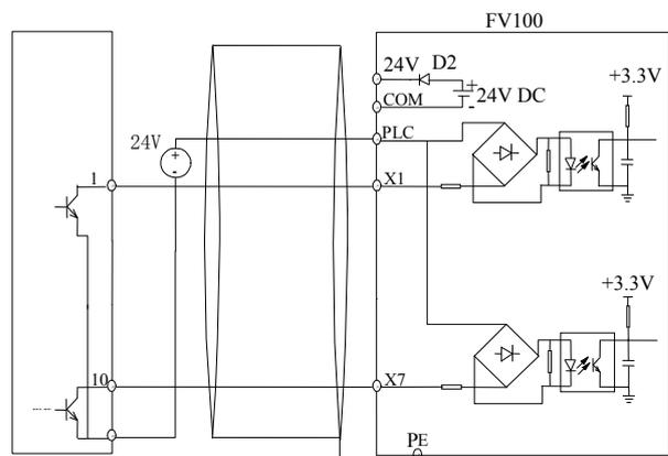
Shielded cable's end near the drive should be connected to the PE
