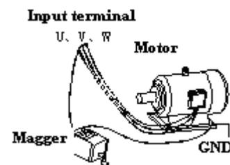
Fig. 1-1 checking the insulation of motor
