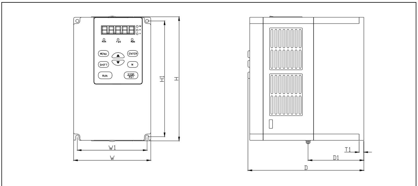
Fig 2-2 FV100-5T-0037G/0055L and lower power VFD
