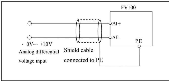
Fig 4-4 AI+, AI- differential voltage input wiring
