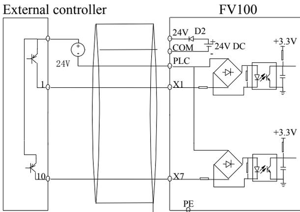
Shielded cable's end near the drive should be connected to the PE
