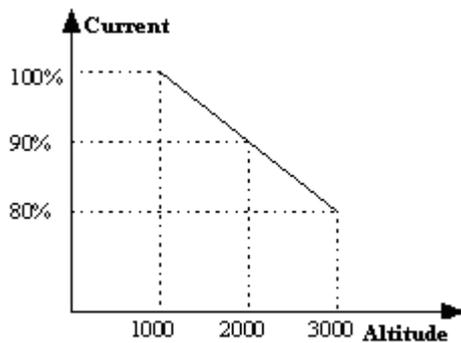
Fig. 1-3 Derating Drive's output current with altitude
