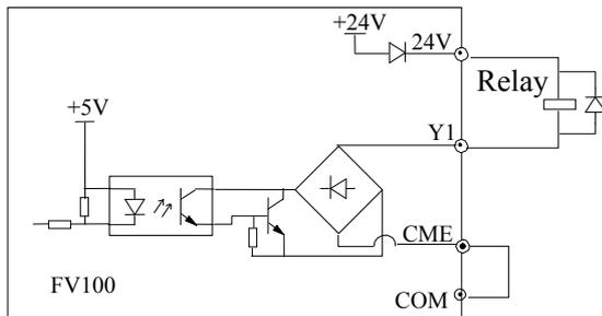
Fig 4-13 Wiring method 1 of multi-function output terminal Y1
