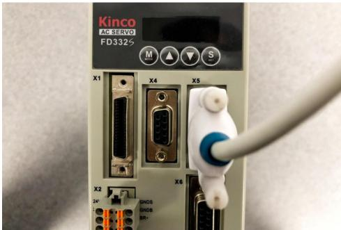
a. For FDxx2S, an RS232 cable (DB9) is required for the X5 connector.
