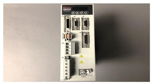
2. With the power disconnected, connect the power wires to the input terminals.
