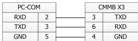
Figure 10-1: Communication wiring between PC (DSub 9-pin) and CD423 controller
