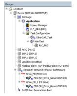
We need to set the Encoder Resolution to match the Servo Drive
