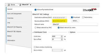
We want to use a Cycle time of 2mS (2000us) so we need to make sure that this is set in the EtherCAT properties
