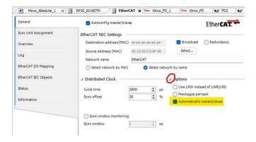
Since we are going to connect to 2 FD Servo drives, we need to make sure that the following addresses are set as shown below using KincoServo+ or KincoServo3
