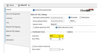
We also want to expand the Options Selection and click on Automatically restart slaves. This will reconnect the EtherCAT devices without having to power down the AK840M if the power is reset on the FD Drives (this takes about a minute to reconnect after power cycling the FD Drives)
