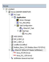
To control the Servo with Codesys Commands we need to add Soft Motion CiA402 devices to each drive
