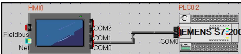
Configuring HMI COM0 client communications parameters: [HMI Attribute]-[COM0 Setting] set the serial communication parameters
