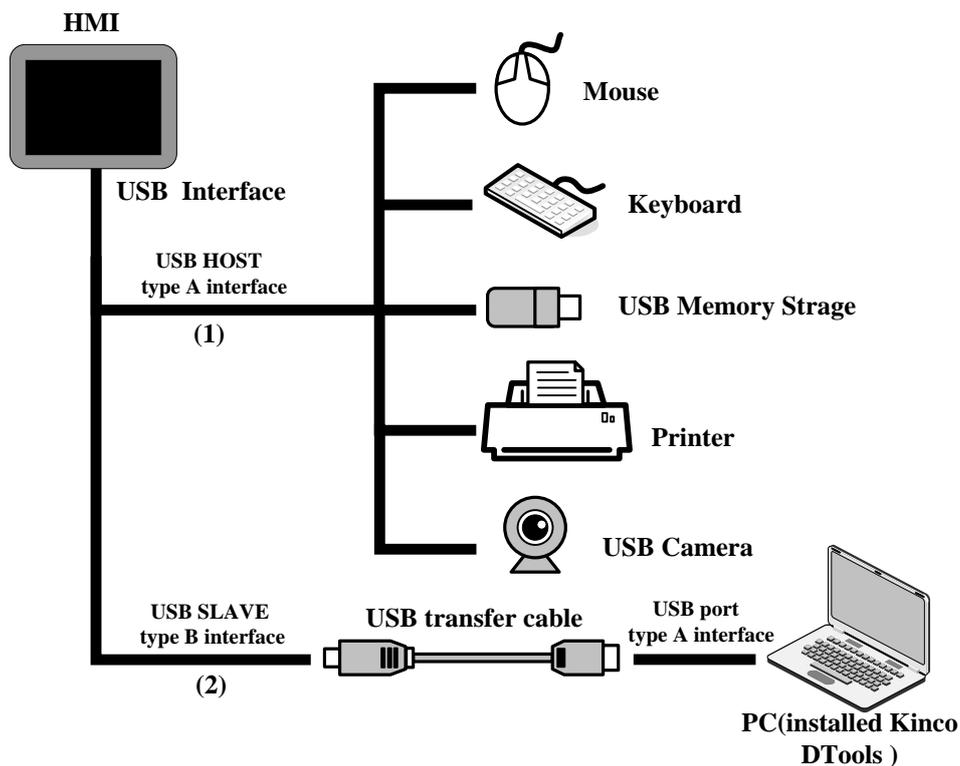
(1) Connect with USB mouse, USB keyboard and such equipments via USB HOST
