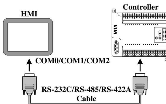
[Example] Below a GH070E with a SIEMENS S7-200 communication, for example, requires the HMI monitor PLC M0.0 output state. (This example uses the HMI COM0 port to connect PLC communication)
