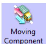
The Moving Component can change the display state and position according to the value of HMI register or PLC register.
