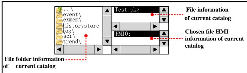
File list component is a special component; it is usually used together with the Import/Export function of Function Key.
