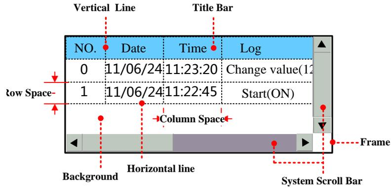
\* When the operation log cannot be wholly displayed in vertical or horizontal direction, system will provide scroll bar automatically. The width of system scroll bar can be set in HMI Extend Attributes of HMI Attributes, the width are optional from 20 to 120(pixel).
