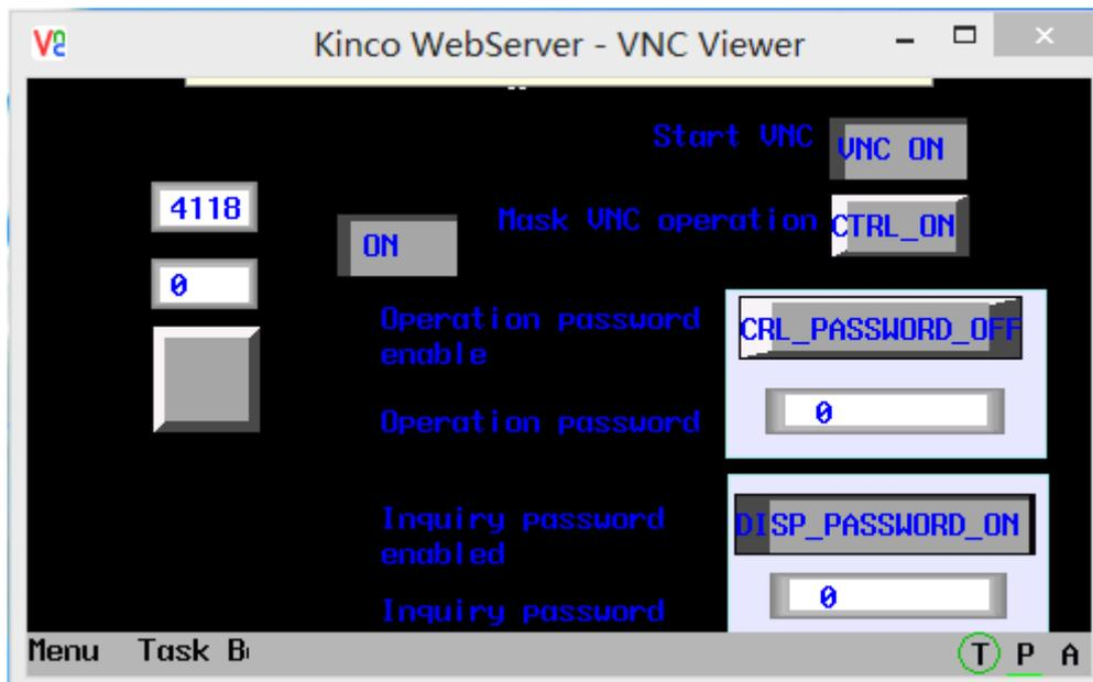
Changes on HMI is displayed on PC simultaneously, meanwhile, user could control HMI by operating on PC.
