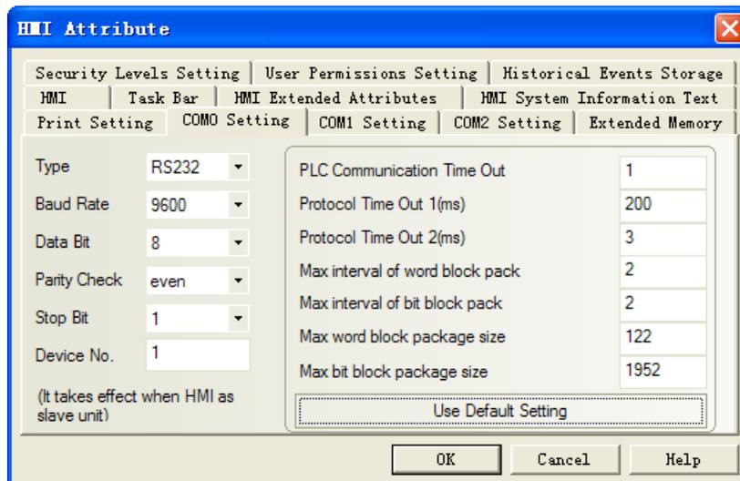
Then from the device number for the HMI station number, other communications parameters set according to specific circumstances.
