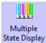
The Multiple State Display Component displays the mapping state according to the value in the specified HMI register or PLC register. It supports at most 256 mapping states.
