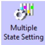
The Multiple State Setting component defines a touch area, if this area is active, this component writes a setting value to an internal specified word register address in HMI or PLC. The display status of component will not be changed by the write values.
