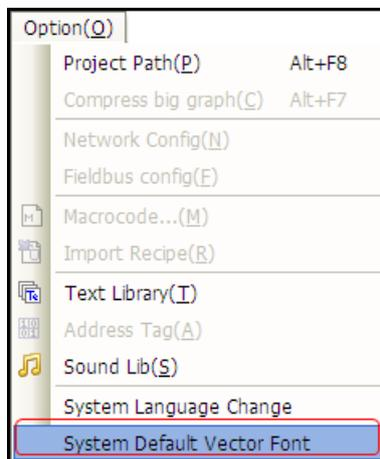
[Example] Set System Default Font as “Arial” , when using tag or text and select “Vector Font” , it will select “Arial” by default automatically.
