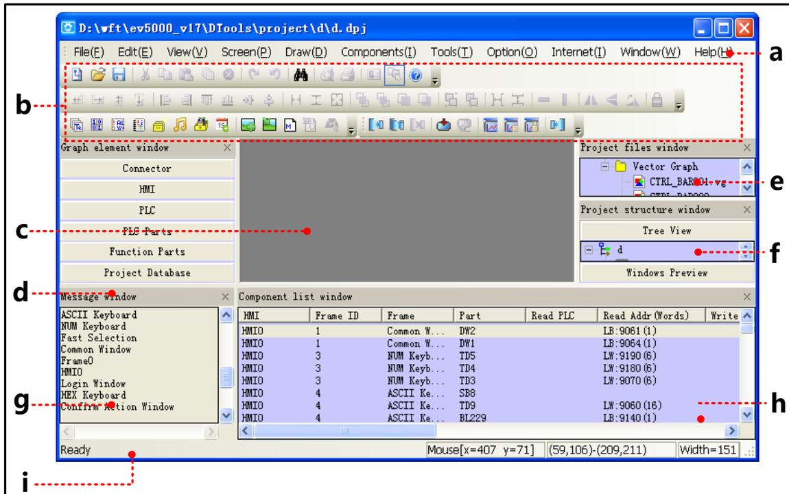
a. Menu bar   b. Toolbar   c. Configuration edit area   d. Component library window   e. Project file window   f. Project construct window   g. Compile information window   h. Component list window   i. Status bar
