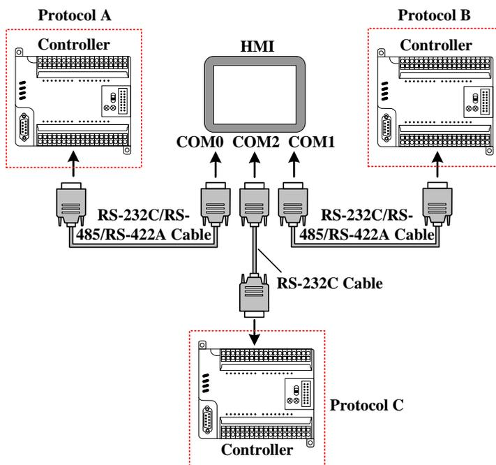
[Example] Below a GH070E with a SIEMENS S7-200 (hereinafter referred to as PLC 0), a MITSUBISHI FX2N (hereinafter referred to as PLC 1), a OMRON CP1H (hereinafter referred to as PLC 2) communication, for example, Requirements were monitored on the HMI PLC 0 of VW 100, PLC 1 of D100 data and PLC 2 in Q 0.0 outputs.
