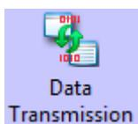
Data Transmission component transmits data in specified HMI or PLC/controller registers to the other HMI or PLC/controller registers. The transmission can be triggered by touching or change of specified register.
