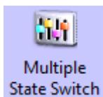
The Multiple State Switch is the combination of Multiple State Display and Multiple State Setting. It displays the mapping status according to the value of Read Address (the maximum mapping status is 768). At the same time, it defines an area, when this area is touched, this component writes the mapping value to the Write Address. The Write Address and Read Address can be the same or different.
