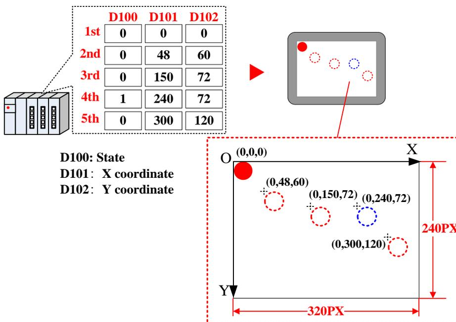
The default word length of Moving Component is 3, each word corresponding to the different control function, see the details follows:
