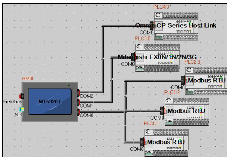
In the [HMI Attribute] - [Serial 0/1/2 setup] According to the serial communications port of the connected PLC actual parameters were set to HMI serial communication parameters, the parameters are set as follows :
