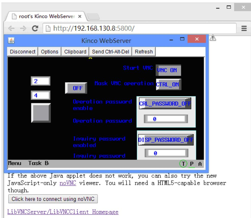
Changes on HMI is displayed by browser simultaneously, meanwhile, users could control HMI by operating on browser.
