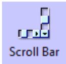
Scroll Bar is used to change the value of HMI or PLC register by moving the slider, and the scaling relation between actual value and Min/Max is displayed by the position of slider.
