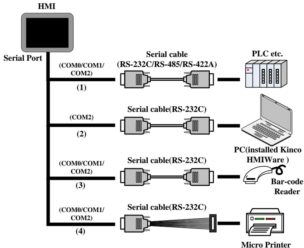
(1) Connect with PLC and other controllers via serial ports to communicate
