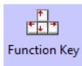
The Function Key provides functions like Switch Window, Keyboard Function, Clear Event, Touch Calibration, save Screenshot to Extended Memory, Execute Macro, and Print and so on. It also can be used to design the key board, and Function Key does not have control register, it executes functions by touch.
