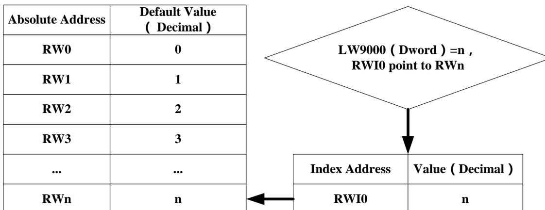
[Example] If the value of LW9000 is equal to 105, then the RWI0 will point to the data in address RW105.
