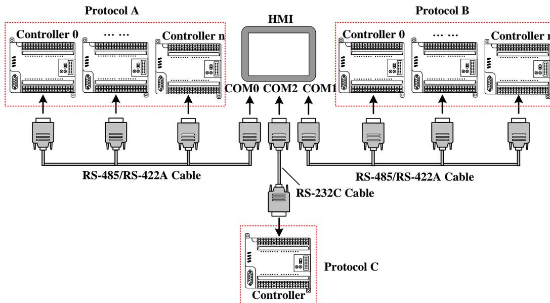
[Example] Below a GH070E with three MODBUS device (hereinafter referred to as PLC 0, PLC 1, PLC 2), a MITSUBISHI FX2N (hereinafter referred to as PLC 3), a OMRON CPH (hereinafter referred to as PLC 4) communication is cases, Requirements were monitored on the HMI PLC 0, PLC 1, PLC 2 of 4X 100, PLC 3 of D100 data and PLC 4 of Q 0.0 outputs.
