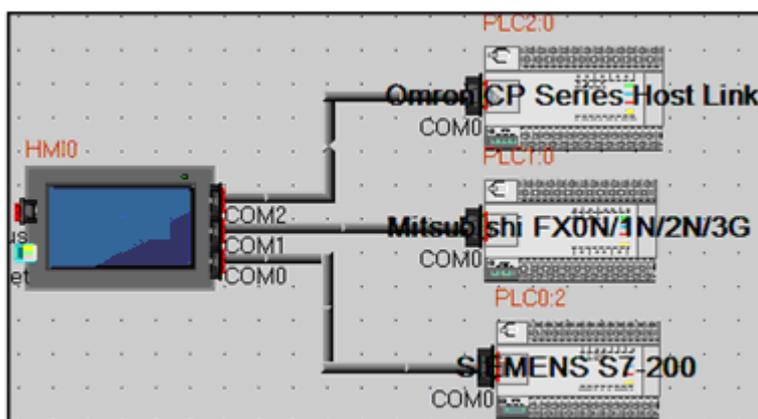
In the [HMI Attribute] - [COM0/COM1/COM2 Setting] According to the serial communications port of the connected PLC actual parameters were set to HMI serial communication parameters, Parameters are set as follows:
