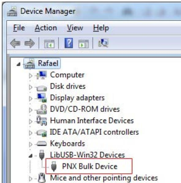
Once the faulty HMI driver is located we can continue to load the proper Kinco HMI USB Driver. Right click on the PNX Bulk Device and select Update Driver Software.
