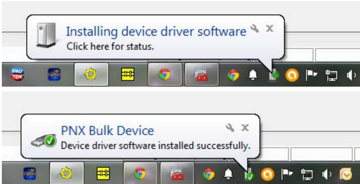
If the developer attempts to download the program to the HMI (via USB) without updating the driver, they will receive a USB handle failed to open error. This error message indicates that the HMI is not powered on or the wrong driver was installed.
